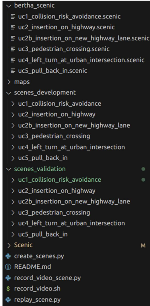
Figure 3.2.1. Structure of the directory containing the “.scenic” and “.scene” files. We can see how the executable scenarios (”.scene” files) are split into development and validation. Inside each “uc” directory, the scenarios are also distributed in different subdirectories corresponding to CARLA’s towns (see Figure 3.2.2). A README.md explains the relevant installation and usage details.
