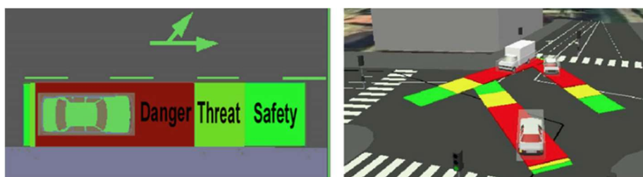
Figure 5. The “Envelope-Zones” of COSMODRIVE model, used to assess path conflict and to manage interactions with other road users (from Bellet et al; 2012)
